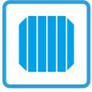
Advanced surface treatment, less surface reflection and 5BB cell design can reduce the series resistance and improve the module efficiency
